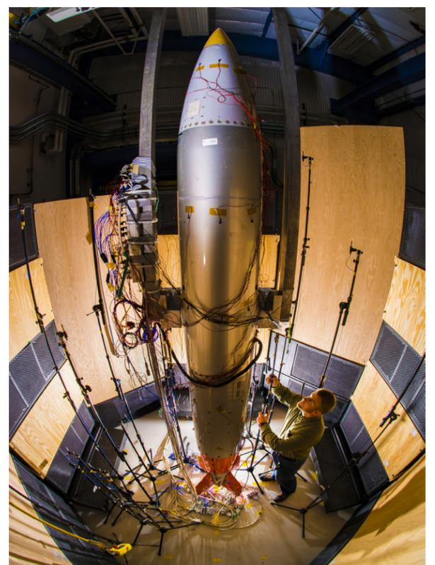
A Sandia National Laboratories mechanical engineer adjusts a microphone for an acoustic test on a prototype of the new B61-12 nuclear bomb, scheduled to go into production by 2020. Photo by US Energy Dept.
