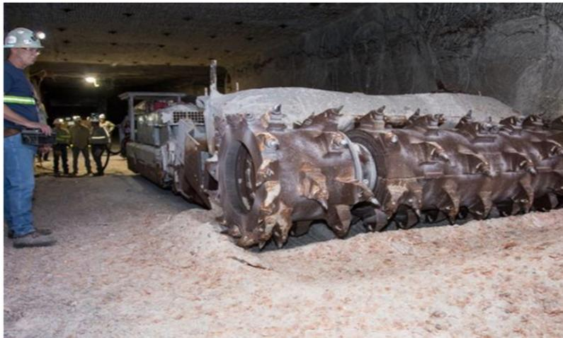
**A heavy grinder gouges into a deep underground salt bed making room for plutonium contaminated nuclear weapons wastes at the damaged Waste Isolation Pilot Plant (WIPP), near Carlsbad, New Mexico. (Photo: Nuclear Waste Partnership, Inc.)**
